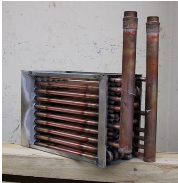
Figure 7.4 Heat exchanger that can be applied in dusty exhaust air
