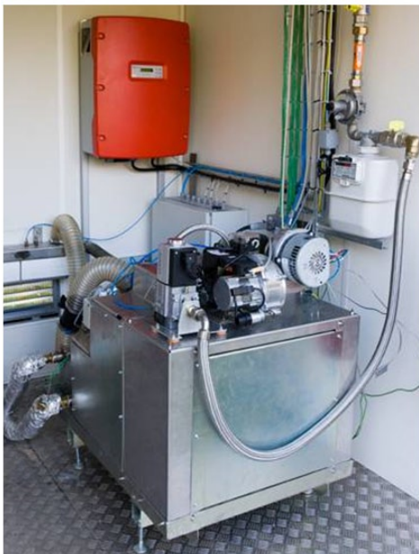
Compower microturbine prototype (left) at field test site with converter to be replaced (red box). Connection to LV network through decoupling inductance (right).
